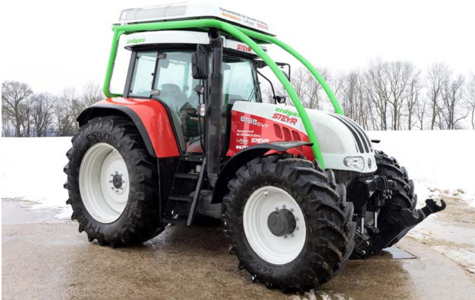
Europe's first diesel tractor – a Steyr CVT 6195 prototype – powered by natural gas / biogas
